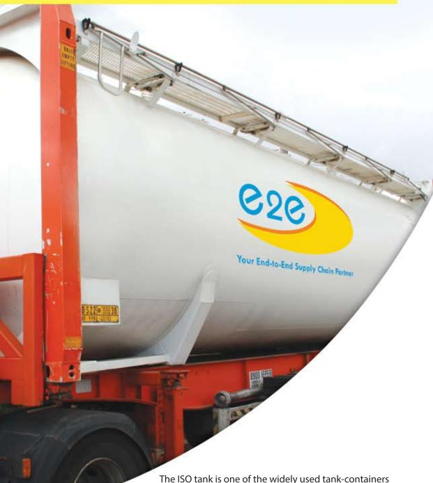
The ISO tank is one of the widely used tank-containers by Chemical, Sugar and Oil Industries for the transportation of hazardous and non-hazardous liquid cargo. e2e offers a range of world-class bulk logistics services and innovative products, including our own fleet of ISO tanks.
